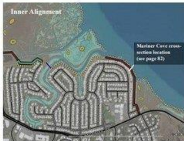
Figure 3.7. Graphic representing a potential inner levee alignment and tide gate designed to protect Mariner Cove and Marina Village.
